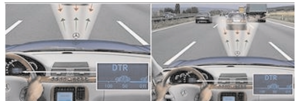
Fig. 5 The Distronic's radar antenna covers all three lanes
