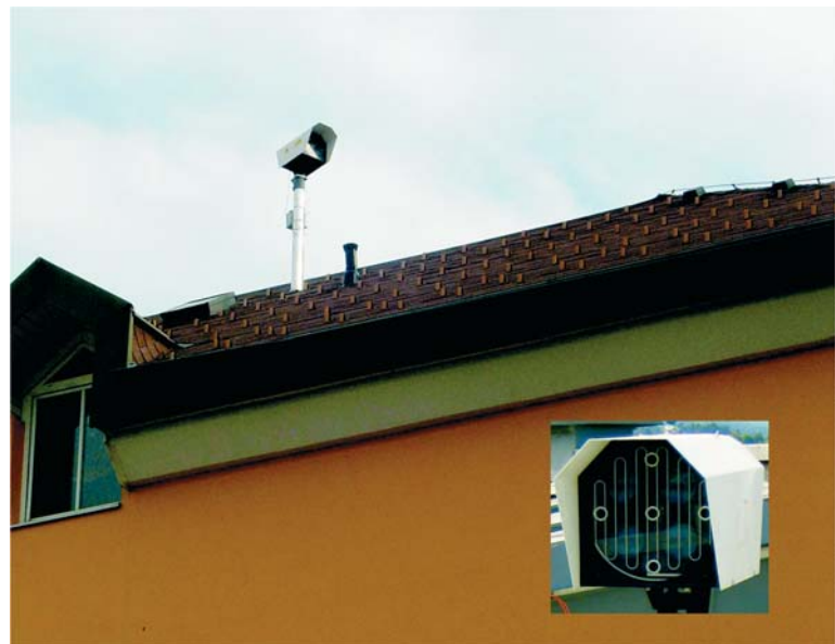
Fig. 2 FSO unit mounted on a roof, detail front view
