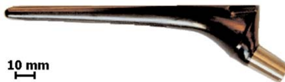
Fig. 5 Optical image of CN_x layer on hip replacement joints
