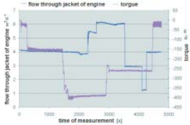
Graph 13(left) Changes in flow through the ICE block and engine loading (that is why the values are negative)
