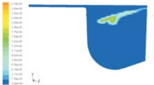
Fig. 29 Droplets of ethanol (kg/s) -10^\circ CA before TDC, kinetic model
