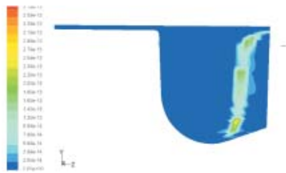
Fig. 32 Droplets of ethanol 5^\circ CA after TDC, kinetic model
