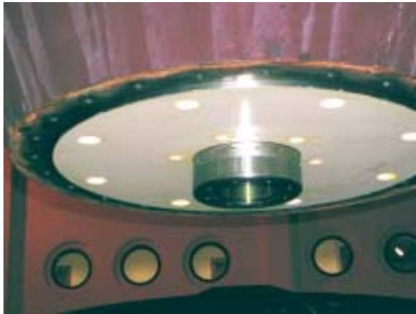
Fig. 1 The rod extrusion from bottom bearing
