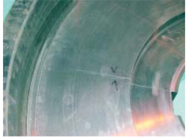
Fig. 8 The crack in the piston of the servomotor
