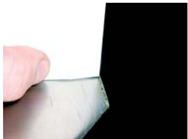
Fig. 6 Extruded material on the edge of the vane
