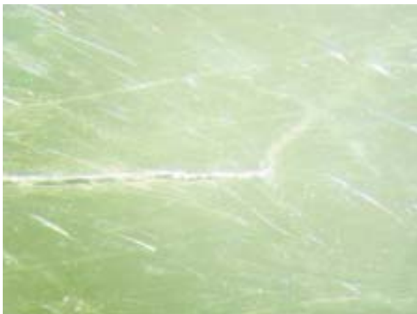
Fig. 9 The detail of the crack end on the piston
