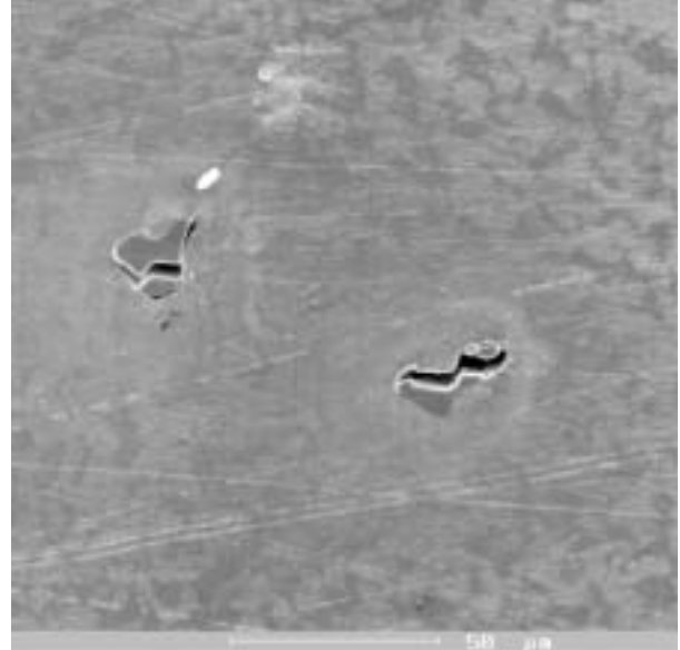
Fig. 16 Cracked inclusions on the surface of the testing rod, REM
