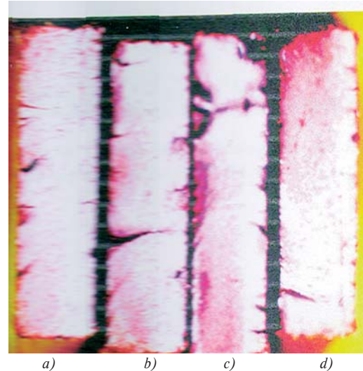
Fig. 10. Fracture surfaces of blasted bars made of steel II 375.1 under flat bending: a) \sigma = 222 MPa, N = 246.200 cycles, b) \sigma = 230 MPa, N = 268.600 cycles, c) \sigma = 209 MPa, N = 733.100 cycles, d) \sigma = 202 MPa, N = 1.405.400 cycles
