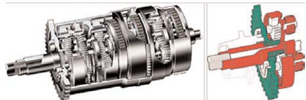
Fig. 1: Agrotron TTV gearbox cross section and detail of the power split point
