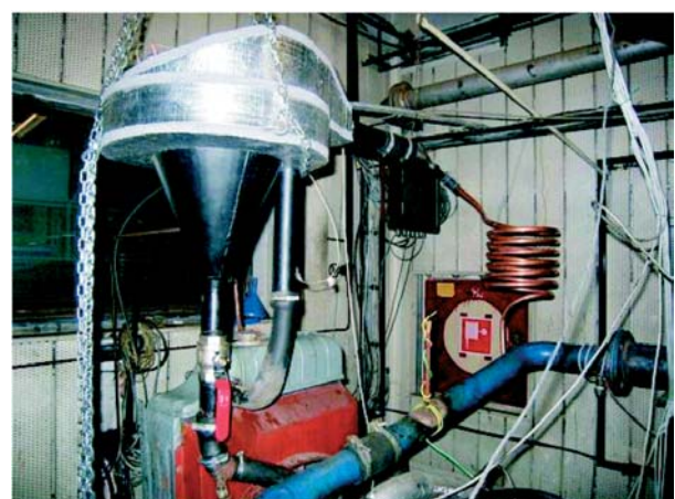
Fig. 1. Flows of energy and part of the conventional cooling system on a test bed [3]
