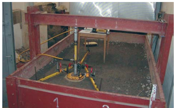
Fig. 5 Static plate loading test in the testing box
