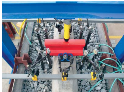
Fig. 2 Measurement of sleeper subsidence under load of rail by hydraulic set ENERPAC with a force of 0 - 50 kN a) scheme b) view
