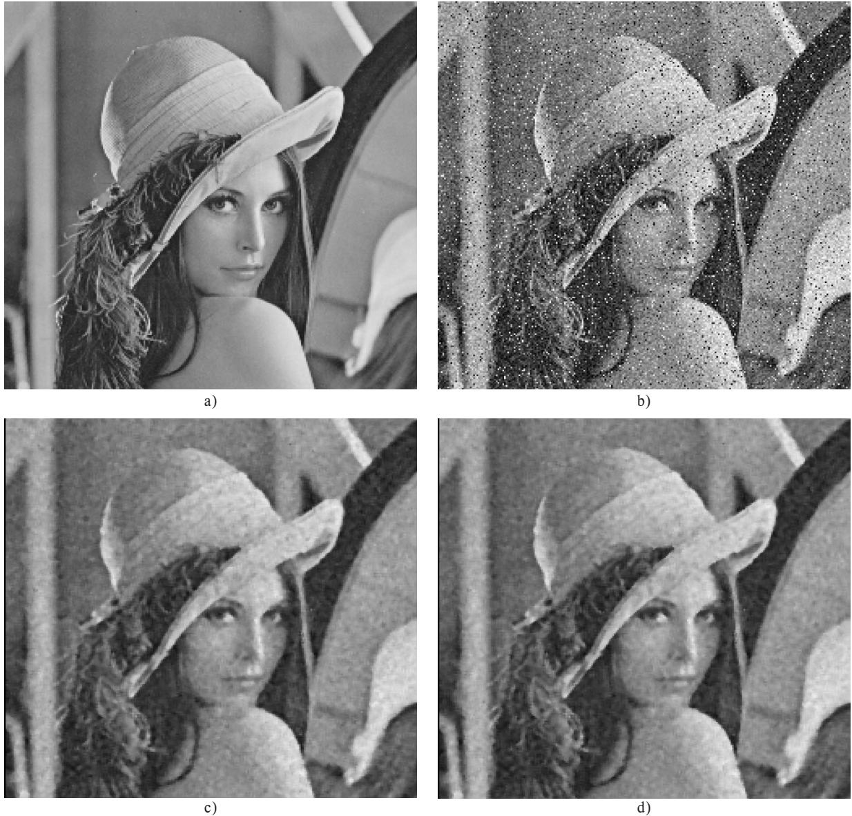
Fig.8 Image Lena, a) original, b) noisy, c) filtered by LMS L-F d) filtered by SMD-SD LMS L-F.
