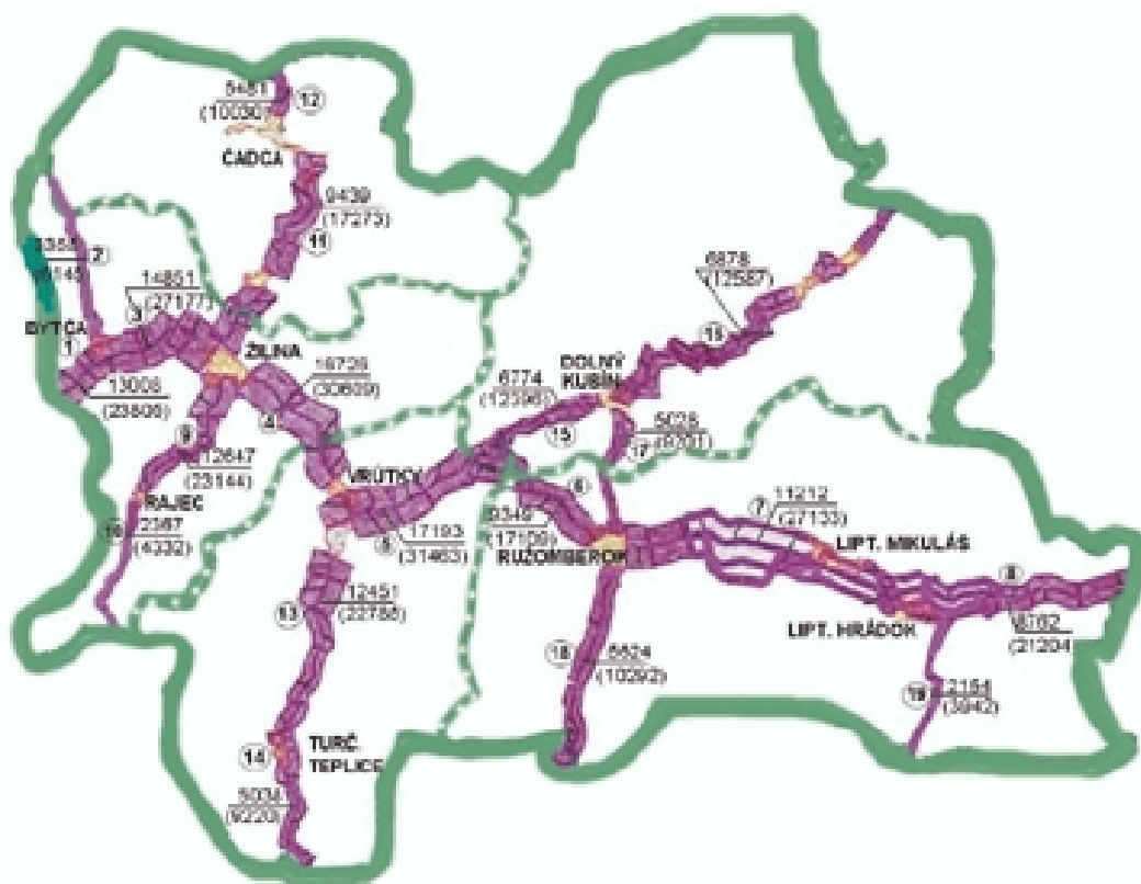
Obr. 2. Intenzita dopravy na cestách I. triedy v sk.v./24h pre rok 2000 (2020) Fig. 2. The traffic volume for 1st class roads in vehicles per day (AADT) for 2000 (2020)
