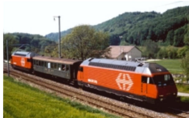
Fig. 10. Test composition (test locomotive SBB 460, measuring coach and braking locomotive SBB 460) during the adhesion tests
