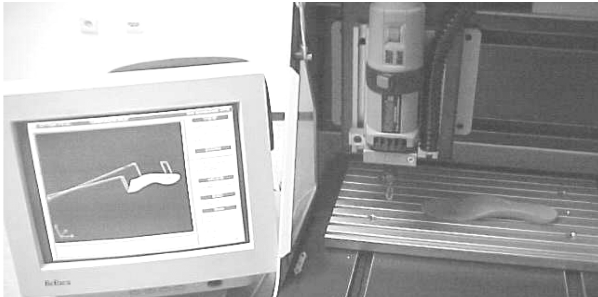
Figure 9. Simulation of cutting tool path generated with postprocessor
