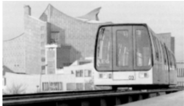
Fig. 1. Maglev-vehicle MAGNETBAHN Berlin [1]
