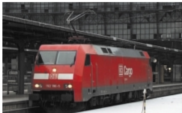
Fig. 8. Class 152 heavy duty locomotive (86 t, 140 km/h, 6.4 MW), which could be equipped with boosters
