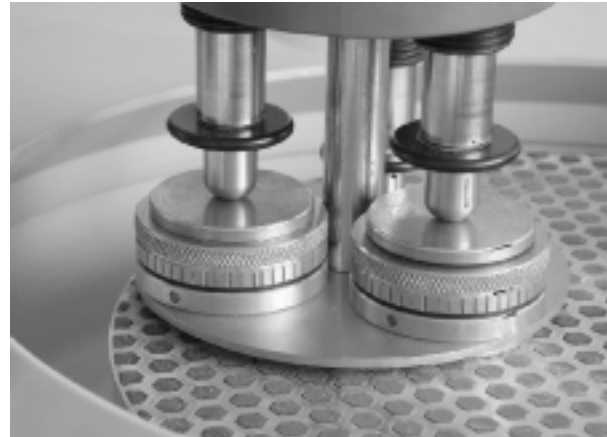
Fig. 4. Metallographic polishing machine with special holders
