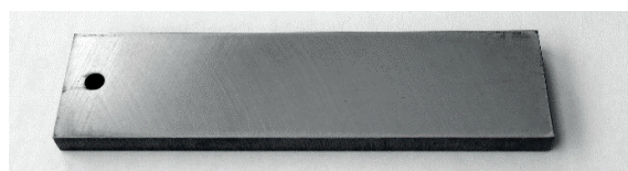
Figure 1 Sample of Domex 700 steel designed both for phosphating and electrochemical tests
