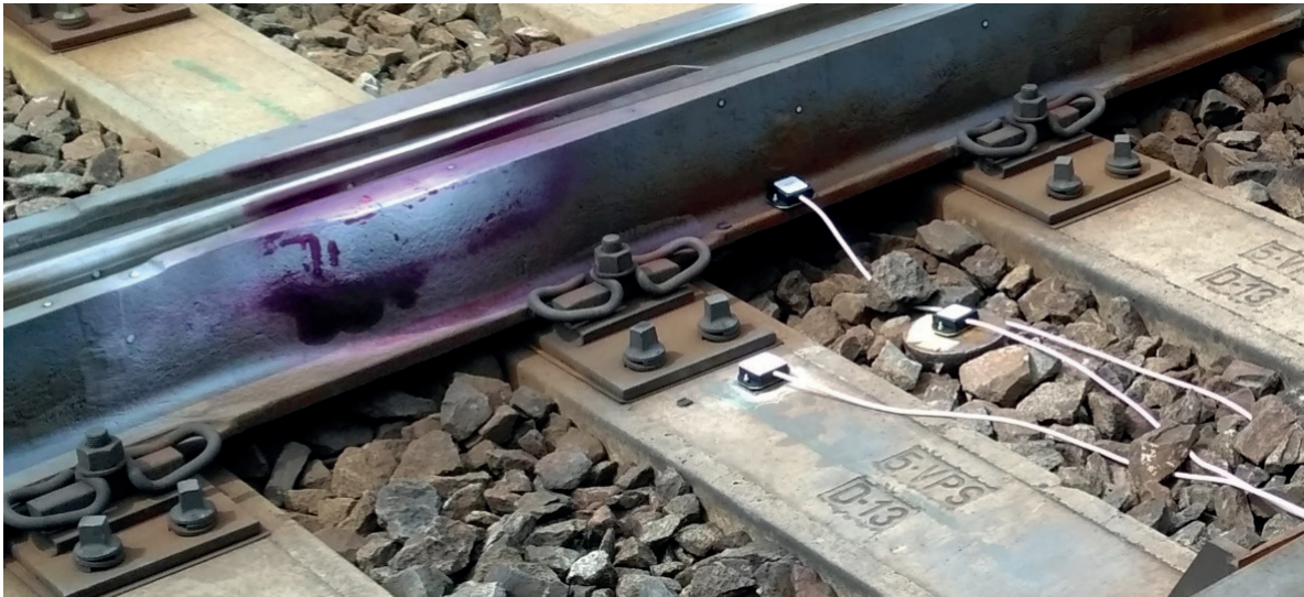
Figure 5 Location of acceleration sensors
