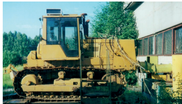
Figure 7 Brake tests of D-160 diesel engine
