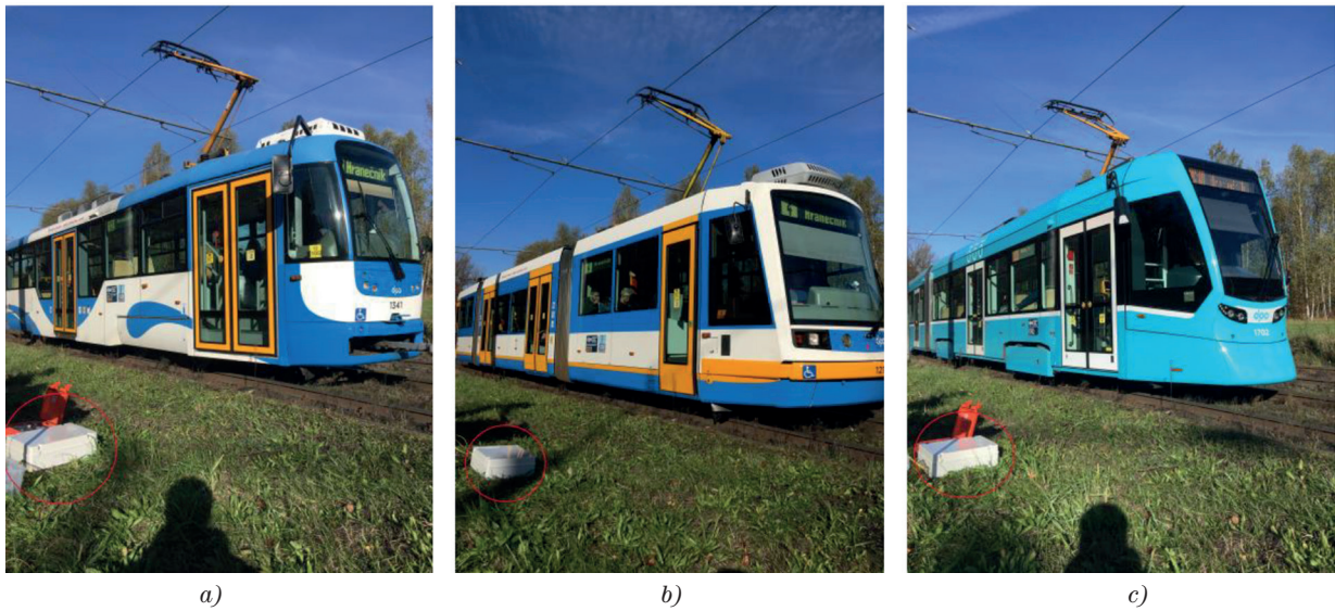
Figure 5 Tram vehicles photos were taken during the measuring process (the red circle labels the position of the sensor)
