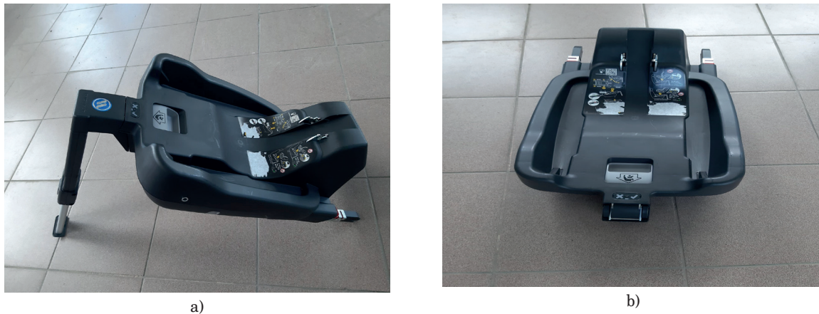
Figure 2 View of the ISOFIX base: a) the base with the stabilizing handle folded out, b) the base with the folded stabilizing handle
