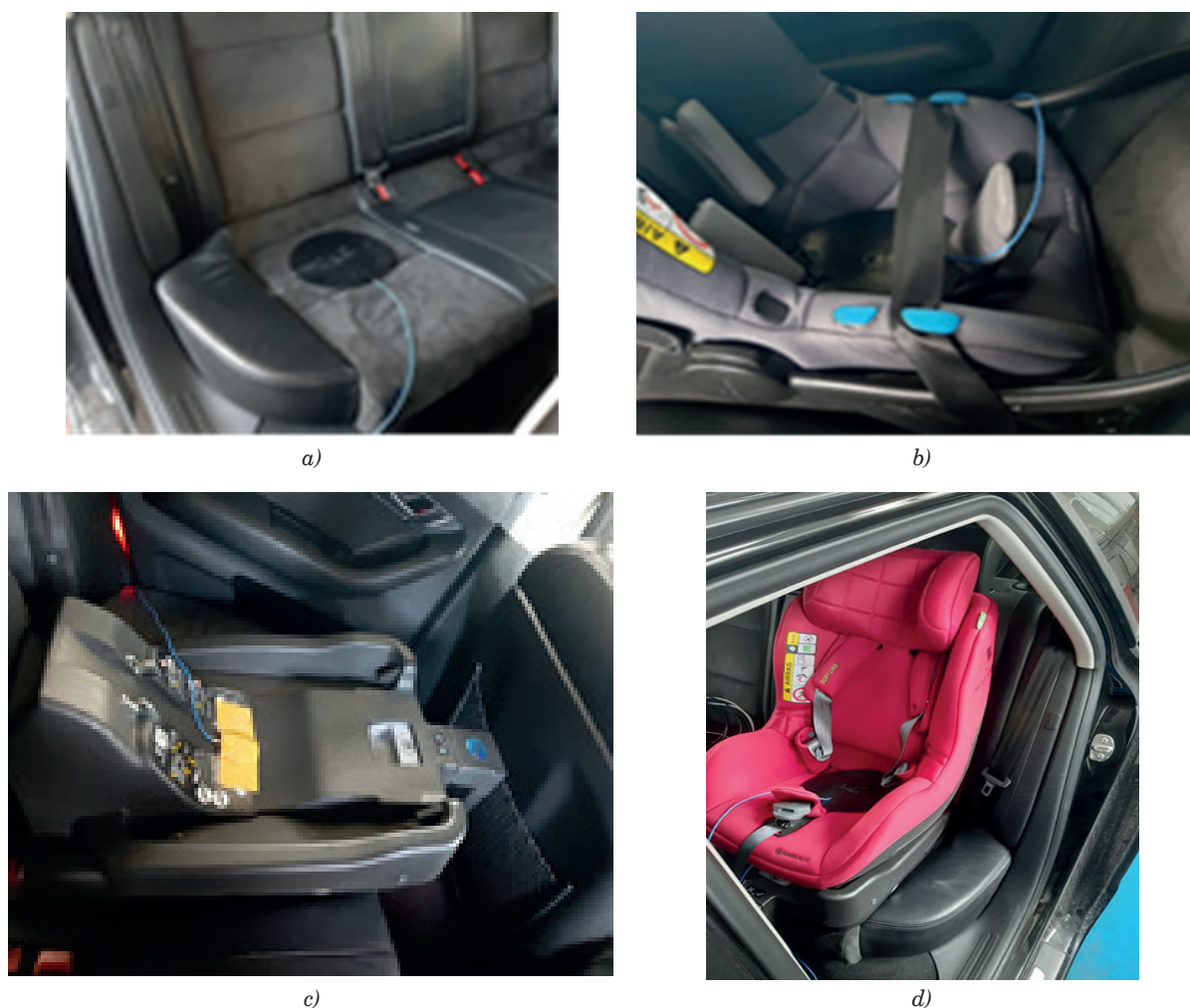
Figure 4 Location of three-way sensors during the testing: a) vehicle rear seat under the child seat, b) the seat child seat (gray), c) ISOFIX, d) the seat child seat (red)
