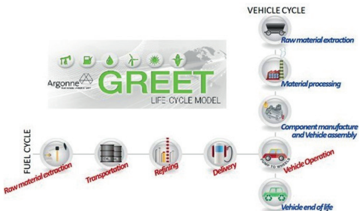
Figure 3 Scheme of the GREET software tool [26]
