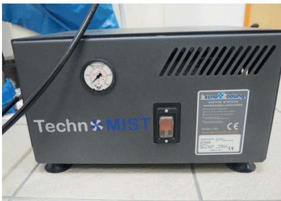
Figure 2 High-pressure pump and filter at the supply line
