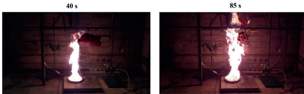
Figure 11 The comparison of gasoline pool fire intensity at the time of 40 s and 85 s from the ignition
