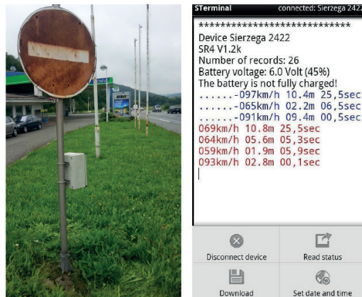
Figure 4 Radar Sierzega, on the left - hand: implementation of the radar on the traffic sign; on the right - hand: the example of reached data from radar [18]
