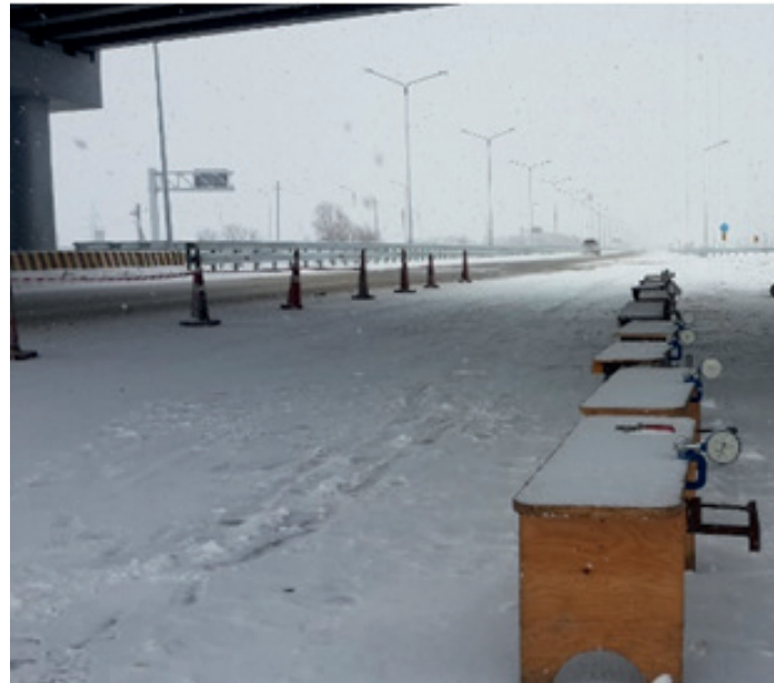
Figure 7 Location of deflection gauges under each of the fourteen beams in the middle of the superstructure No. 1
