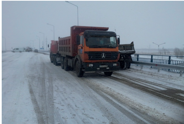
Figure 4 Vehicles are located at the roadway safety fence of superstructure No. 1 from Kapshagai at the first stage of testing
