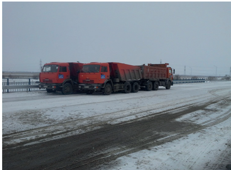
Figure 5 Vehicles are located at the roadway safety fence technical of superstructure No. 1 from Almaty at the second stage of testing
