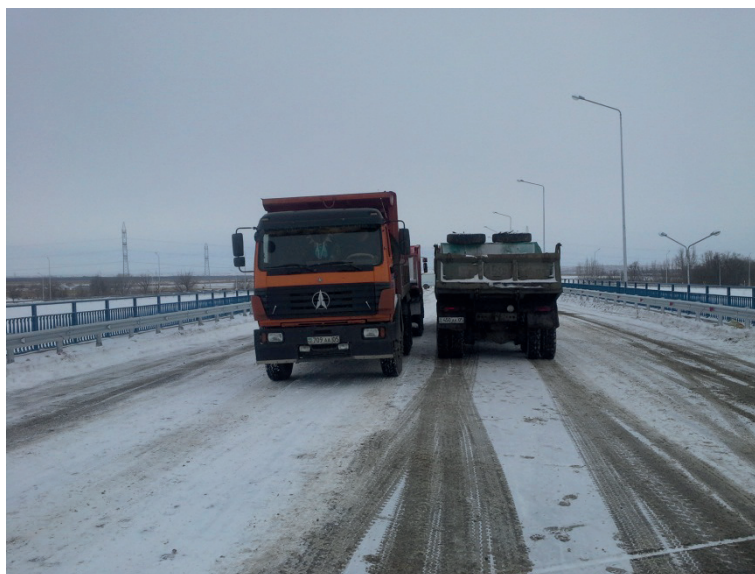
Figure 6 Vehicles are located at the longitudinal axis of superstructure No. 1 at the third stage of testing
