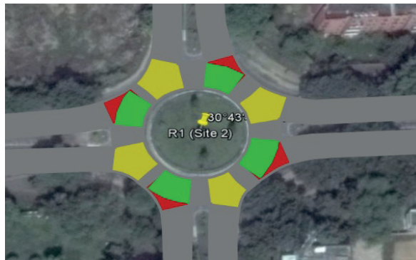
(a) Conflict area settings for R1 and R3
