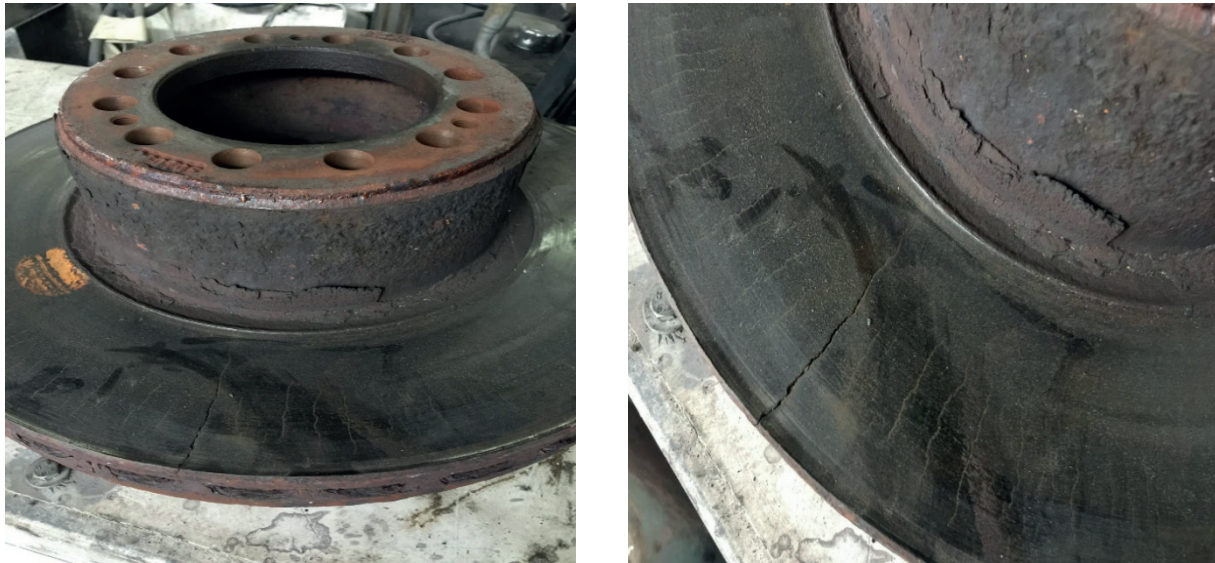
Figure 1 Defects of the brake disk of a truck
