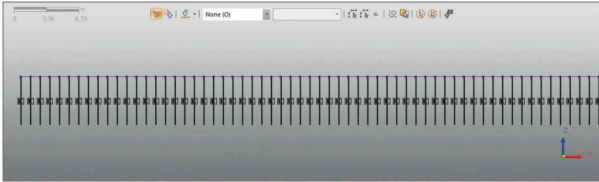
Figure 6 Part of the finite-element model of a beam on elastic foundation
