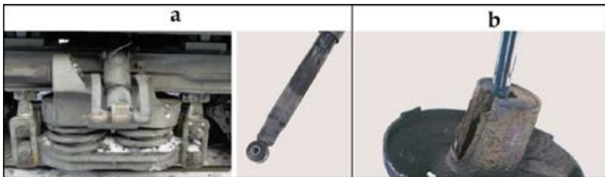
Figure 3 Examples of damaged hydraulic shock absorbers: a) leakage of absorber's oil, b) a broken piston rod
