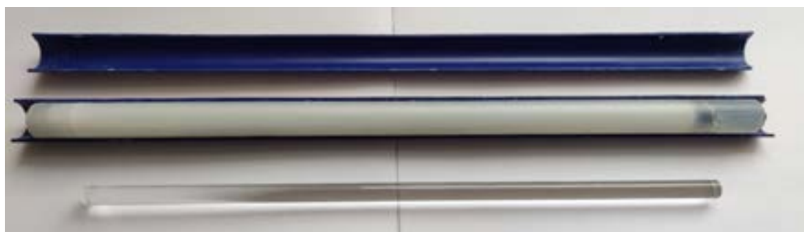
Figure 6 Silicone mould with casting from the PRC1710 material
