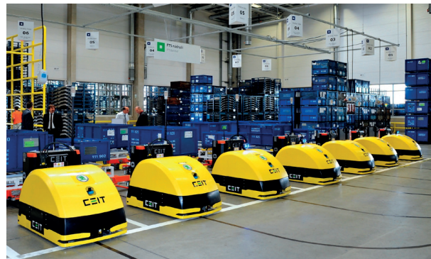
Fig. 10 CEIT logistics system working in automobile industry
