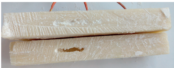
Fig. 9 Shrinkages and cavities in the samples
