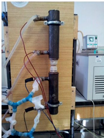
Fig. 2 Experimental device to measure heat flow through GHP with calorimetric method
