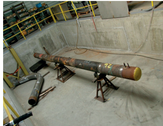
Figure 4 Pipeline with two types of welded repair patches
