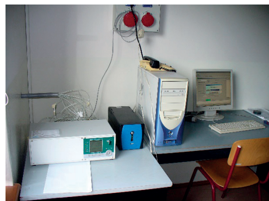
Fig. 6 View at data recording device ALMEMO 5690-2M in the office next to the laboratory rooms (May 2011)
