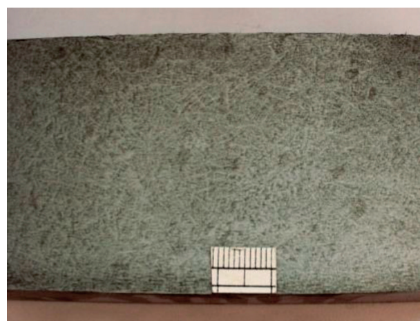
Fig. 3 Macrostructure with segregates
