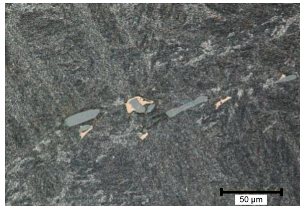
Fig. 6 Microstructure with inclusions
