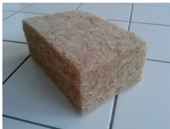
Fig. 8 The representative test specimen of thermal hemp insulation
