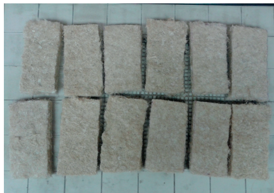
Fig. 9 Two sets of test specimens soaked in the fire retardant
