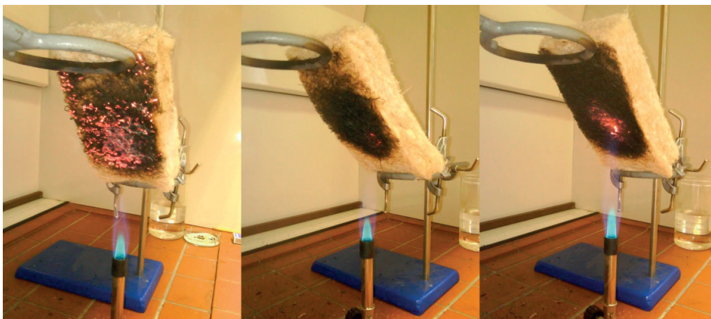
Fig. 11 The test specimen consolidation in holder, flame height measurement, testing (left to right)
