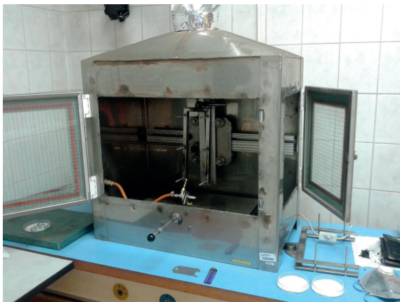
Fig. 2 The test device - combustion chamber located in the fire-chemical laboratory of KPI FBI ZU
