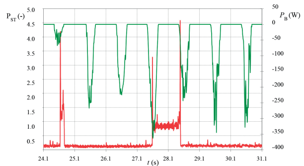
Fig. 3 Flicker and photovoltaic power in the on-grid mode
