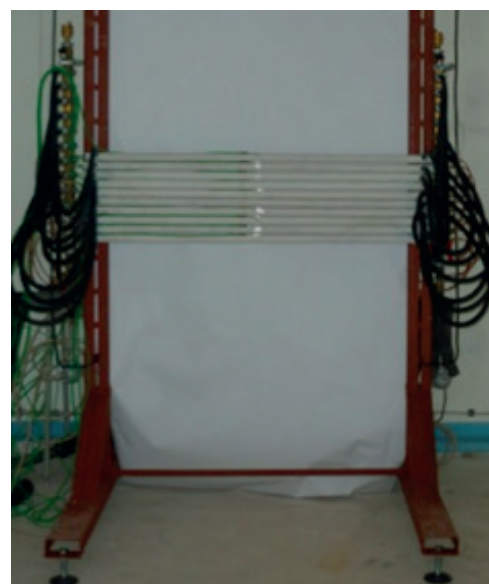
Fig. 3 Arrangement of pipes in a thermostatic chamber at axial distance of pipes 1D [6]
