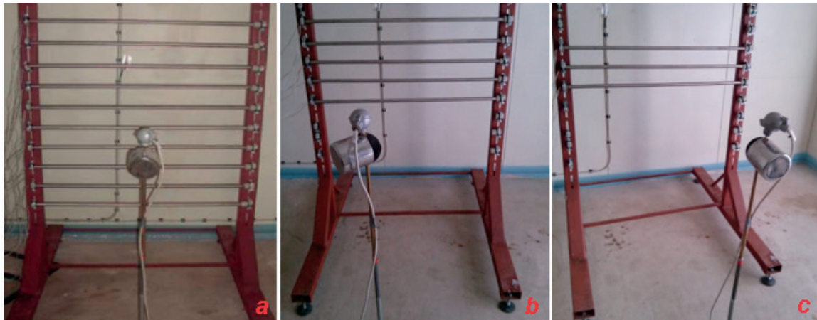
Fig. 5 The fixing of a) ten, b) five and c) three horizontal heated cylinders on the stand in thermostatic chamber
