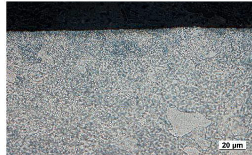
Fig. 3 Microstructure of milled surface, VB = 0.05 mm, HAZ ( 2\mu m )
