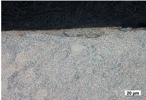
Fig. 5 Microstructure of milled surface, VB = 0.6 mm, HAZ (5 μm)
