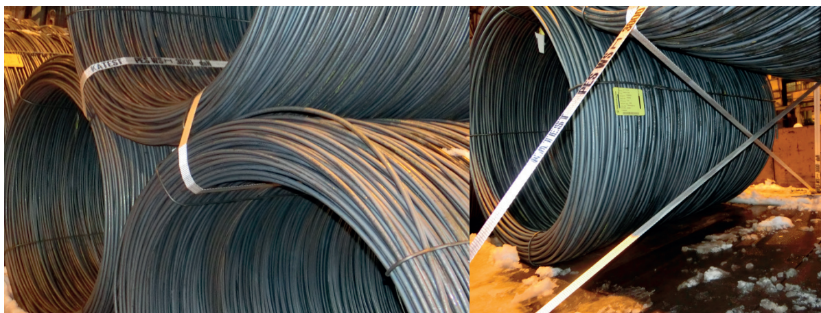
Fig. 1 Securing of the coil in the upper layer in the first series of impact tests (on the left) and in the second series of impact tests (on the right)
