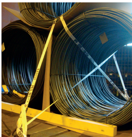
Fig. 3 Lashing on the wagon Rils in the third series of impact tests
