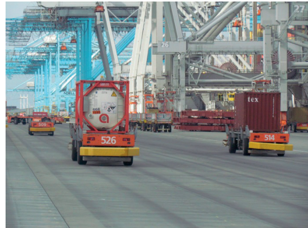
Fig. 4 Automated guided vehicles in ECT Delta Terminal Source: authors
