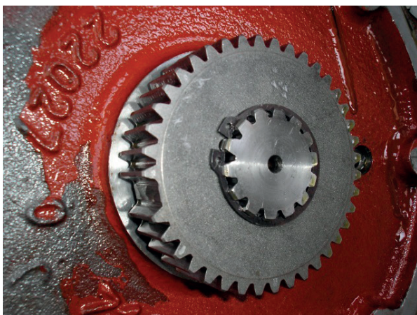
Fig. 6 Sun gear with one missing tooth
