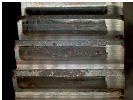
Fig. 3 Sun gear of planetary gearing damaged by artificially created pitting (left) and sun gear damaged by real pitting (right)
