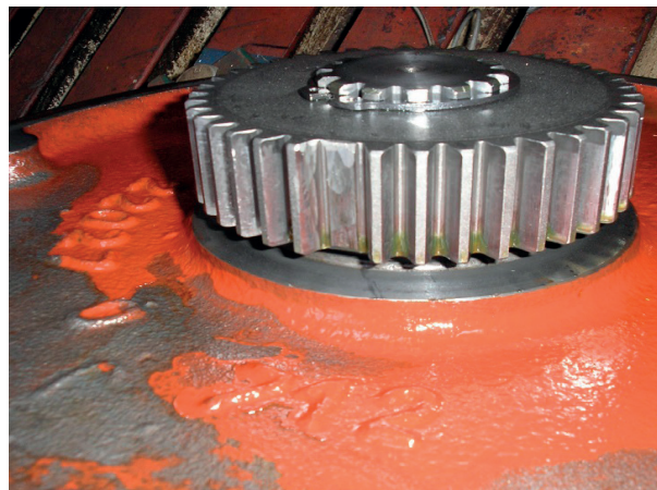
Fig. 6 Sun gear with one missing tooth
