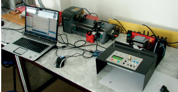
Fig. 12 General view of the workplace verification system and use of standard STEP-NC
