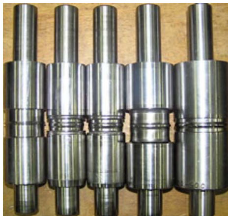
Fig. 6 Thorns on rolling bearing rings
