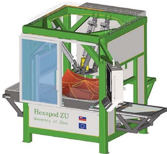
a) The design of machine based on parallel kinematic structure used for high-speed machining or manipulation
