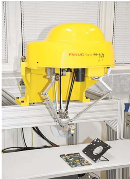
a) Application of delta robot for assembling of electronic device
