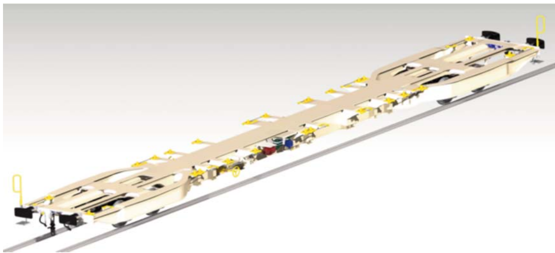
Fig. 2 VEL-WAGON 3D model used for modelling and simulations (Source [6])
