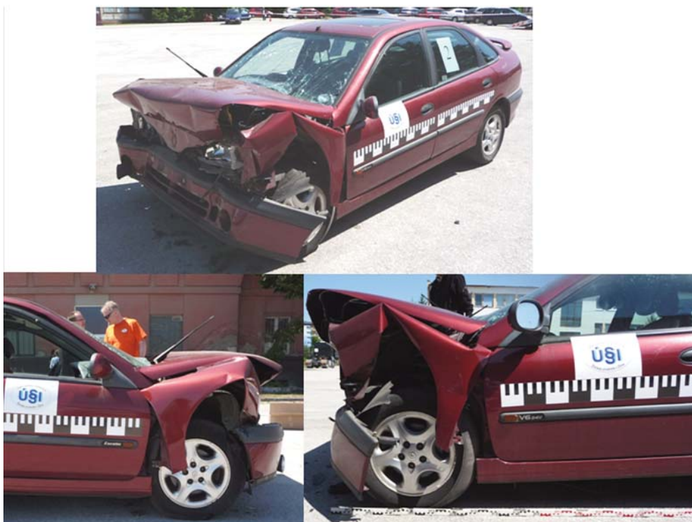
Fig. 5 Damage of the car Renault Laguna (EES = 62 km/h)
