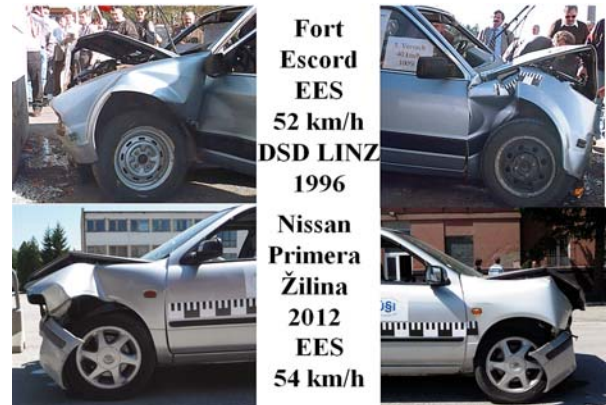
Fig. 17 Comparison damage of cars Ford Escort (Crash tests DSD LINZ 1996) and test car Nissan Primera (Crash tests Institute of Forensic Engineering, University of Zilina 2012) [2]
