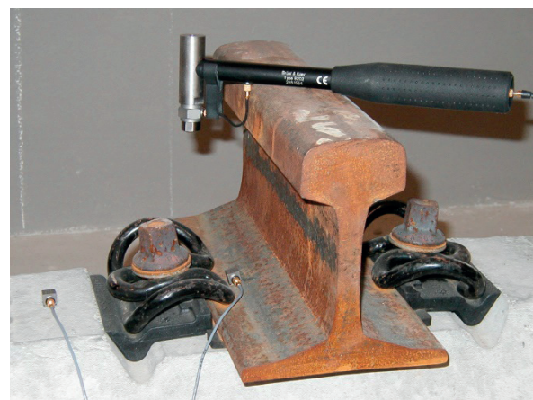
Figure 3 View of the rail fastening sample
